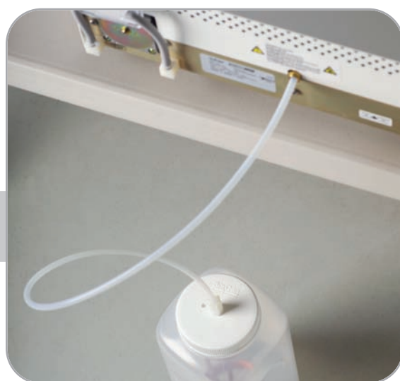
Single Use Water System
